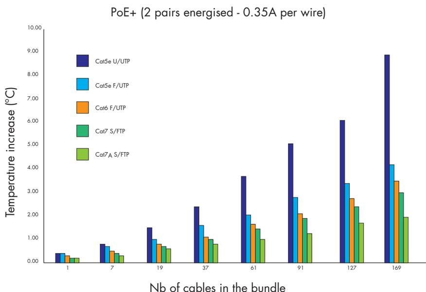
Figure 2: Relationship between bundled number of cables running PoE+ and temperature gains
