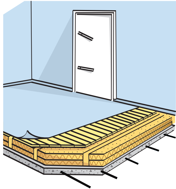
Example of heating cable in freezer floor.
