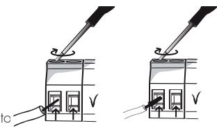
If connecting two or more conductors into the same terminal (regardless of type) do the following: Attach a metal crimp (use crimping tool) over any 0,5 mm<sup>2</sup> conductor(s) and place the crimp(s) covering the conductor(s) into the terminal. Then fasten normally.
